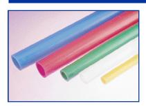
Polyethylene is one of the most popular choices for low pressure tubing due to its resistance to most chemicals and solvents, good flexibility and economical cost. Our PE Tubing is manufactured from high quality resins and extruded to close tolerances. We offer five popular sizes. Compatible with Coilock Fittings (pages 73 - 74) and Poly-Tube Fittings (page 75).
