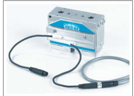
Model SPG300 shown with Code E23C or E24C face mounted, quick-disconnect, electronic sensors.
